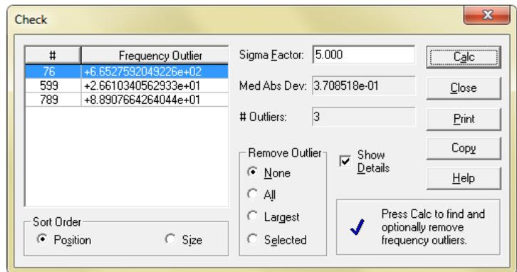
Figure 5. Example of Stable32 Check Function Screen
